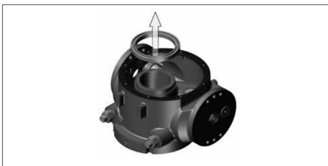
Step 2. Remove yoke top bearing (56) from yoke (13).
