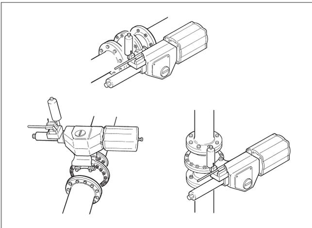
Fig. 7 Ways to install the actuator
