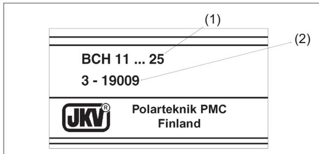
Fig. 4 Information on pump unit identification plate
