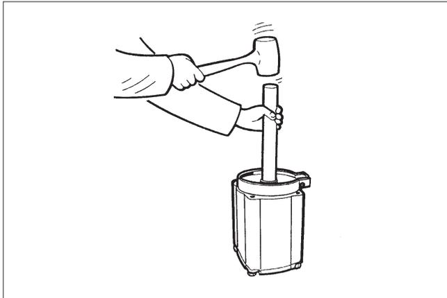
Fig. 19 Placing the piston in the cylinder
