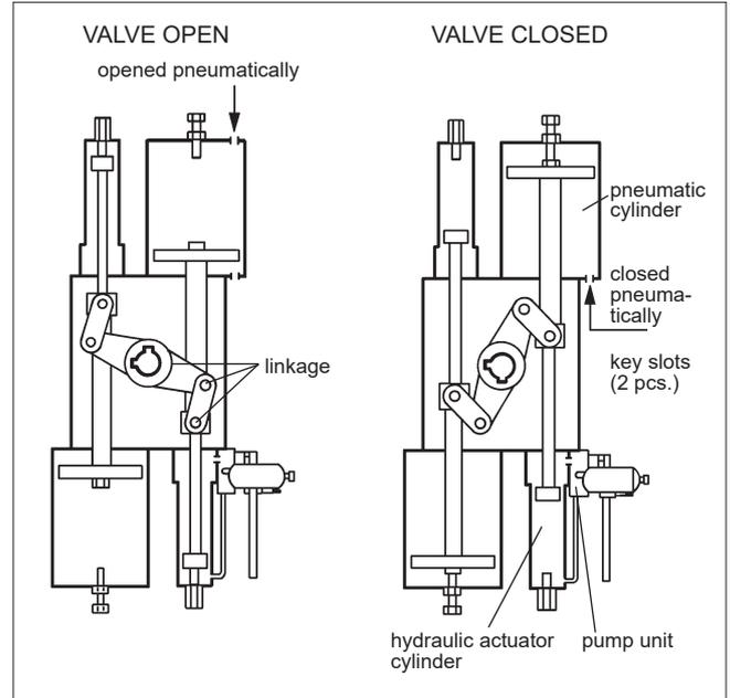
Fig. 2 Operating principle of the B1CH502 and BCH502 actuators as seen from the valve side
