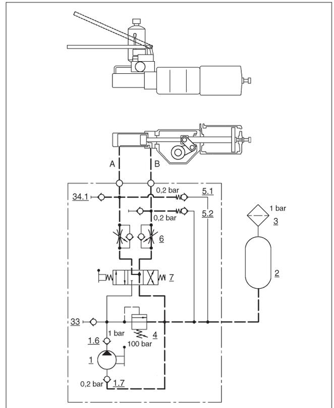
Fig. 11 Operating principle of the hydraulic pump unit on remote control
