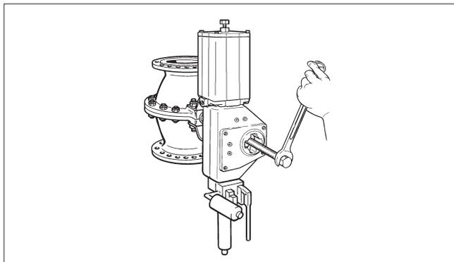
Fig. 9 Removing the actuator with the extractor
