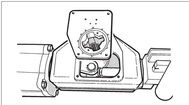
Fig. 20 Mounting the cover on the housing
