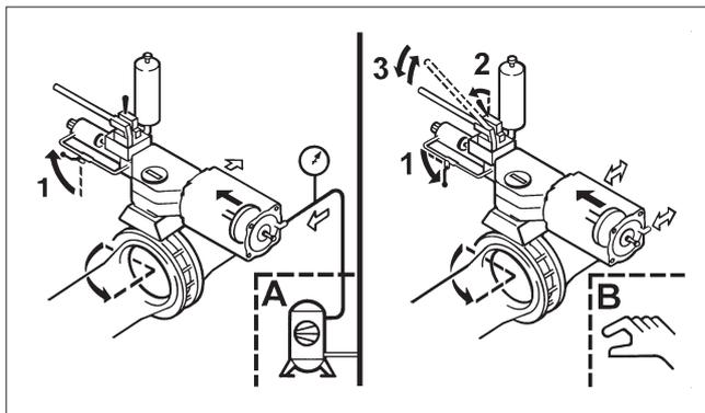
Fig. 14 Operating instructions plate, opening the valve and operating the by-pass valve
