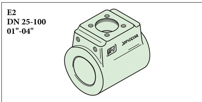
The rigid end-entry type stainless steel body holds the pressure load and pipeline forces protecting the ceramic materials from breakage. The end bushing is screwed to the body enabling easy maintenance.
