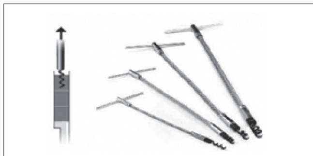
Fig. 13 Typical gland packing removal tool
